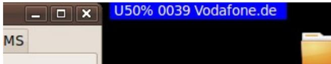
**ixconn** now always displays the current signal strength, the speed of data transfer and the network name. If the transfer speed drops to a level below 0.5 Kilobytes per seconds, then the sum of the transferred data volumes is displayed in its place (four-digit value in units of Megabyte). You can switch to the usual detailed representation via clicking per left mouse click action.
